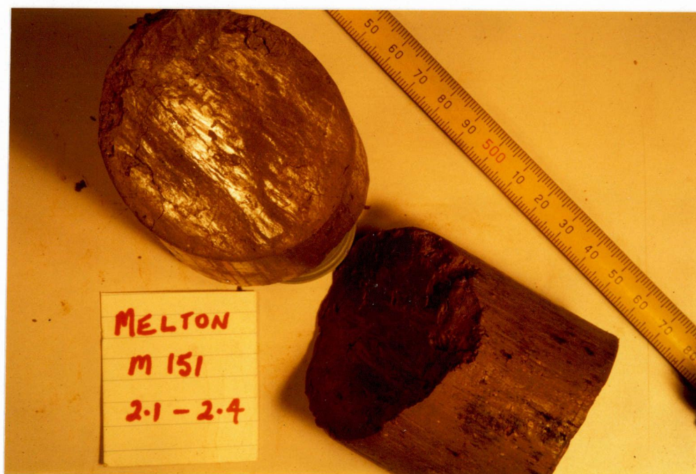
Plate 2 Slickensliding of fissure in soil core.
