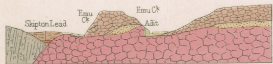
Sketch Section at west boundary of Allot A' Emu Creek, (Looking West)
